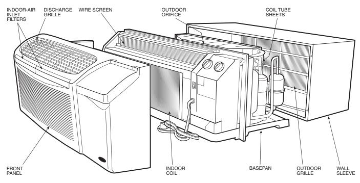
FIGURE 6 — UNIT COMPONENTS
